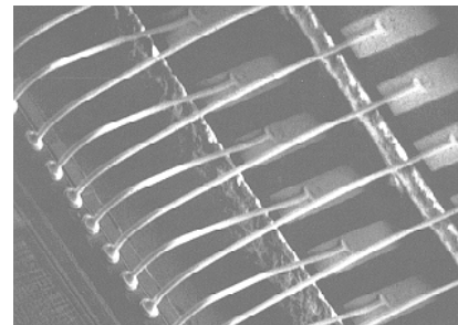
Fig 7. Thermo Sonic ball bonding from die to lead frame
